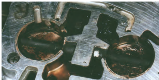
Picture J - Carburetor plates before P.i. treatment
